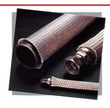
INDUSILRope is used for high temperature packing, seals, core for tadpole tapes, and seals for casting moulds. To improve handling properties during installation, INDUSIL Rope has a coating, which will decompose, at high tempetures. Severe abrasion applications will require other external protection measures.
